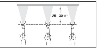
Keep the spray gun at right angles to the surface. This means moving your entire arm back and forth rather than just flexing your wrist.
