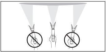
Keep the spray gun perpendicular to the surface, otherwise one end of the pattern will be thicker than the other.
